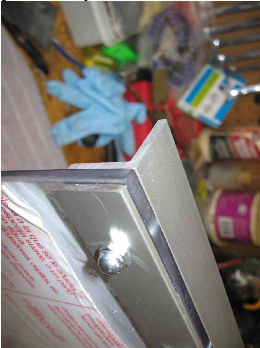
Using the outside 2 holes as pilot holes I drilled through the lexan and the flat aluminium. I then put the bolts and acorn nuts into these 2 holes to keep the pieces from shifting. I went to the center and worked out drilling the remaining holes. I put another nut and bolt in the center hole before drilling the rest.
