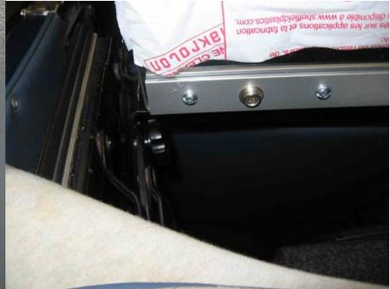
The flat head #6 screw sits flat inside the snap. It will not interfere with the dome piece. You cannot use a pan head here, as it will contact the “rolled over” piece of the dome.
