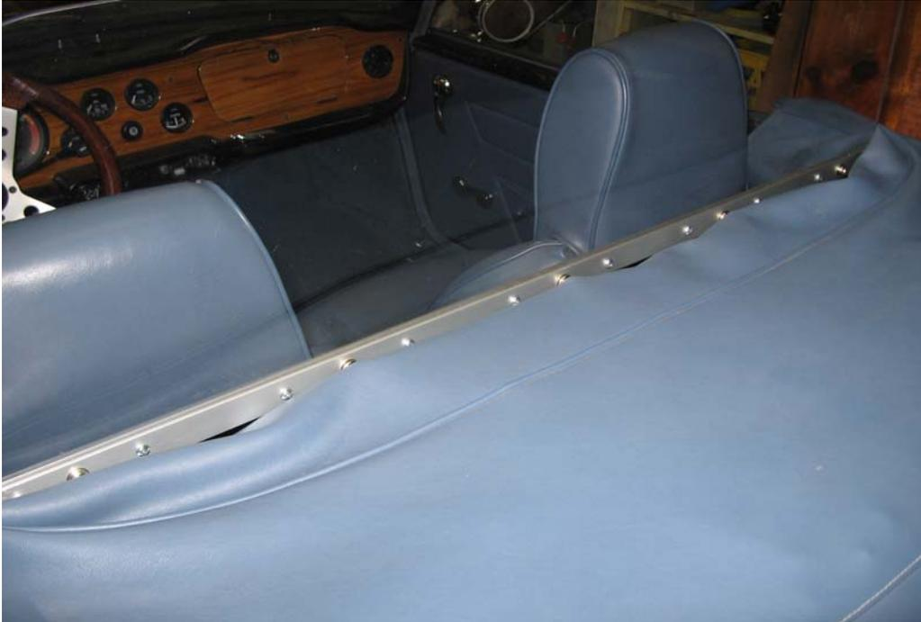
I am not terribly happy with the flatness. I might move the right-pictured dome so as to stretch the material a little tighter to look like the left dome. I have not attached the outside snaps as I want to cut the slots in the soft top cover for the support bracket bar first to see where the soft top finally sits.
