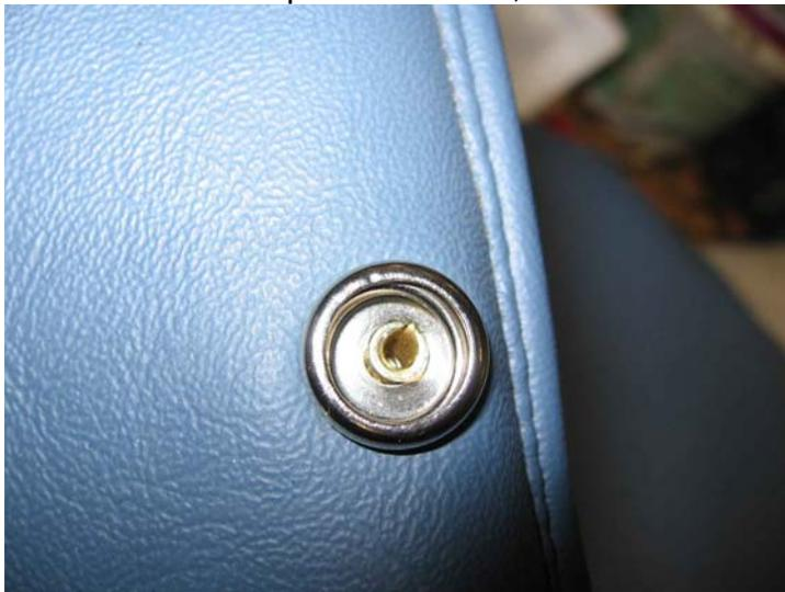
Below are pics of it attached. I had the snaps below the piping on the soft top cover then moved them to 1.5 inches the other side of the piping in order to tighten up the snap location so the soft top cover sat flatter.
