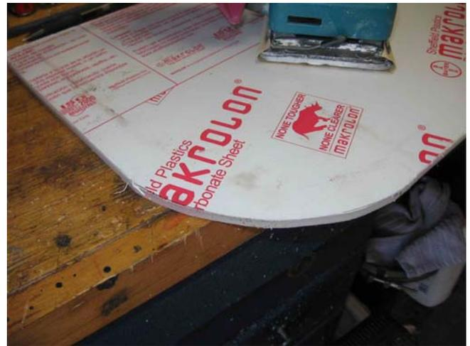
8: I used a vibrating palm sander with good quality sand paper to sand all edges of the lexan. You want to get it very smooth with no "cutting" marks. When I had it clean of all marks and slightly rounded I then started the wet sandpaper sanding. Start with say 300 and slowly work up to a final 2000 all by hand sanding. Use plenty of water so your paper lasts. You can do a final polish with a plastic polish. This stuff is a LOT tougher than plexiglass.
